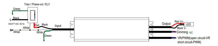
Using 0-10/1-10v wiring diagram (the power does not pass through the dimmer)
